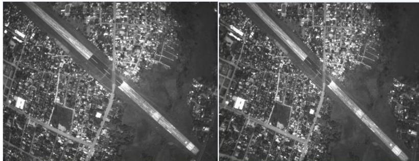
Figure 11. (L-R) Raw LCTF Image and Radial-Lens Corrected LCTF Image
