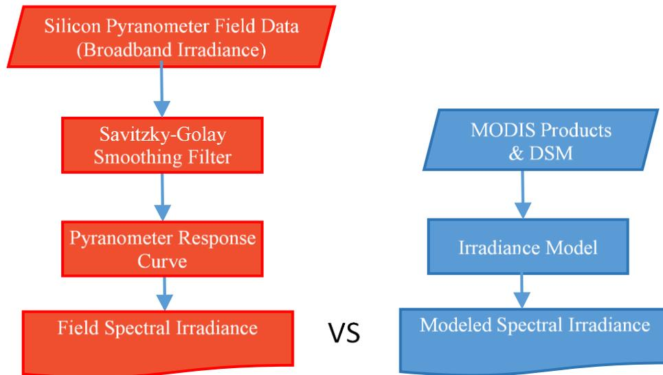
Figure 3. Process Flow of Model Implementation and Validation
