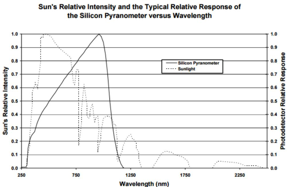
Figure 4. Silicon Pyranometer Response Curve
